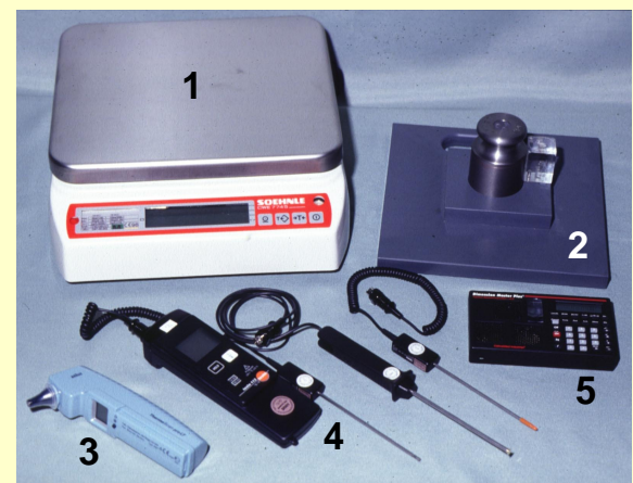
Figure 2. Measuring devices for death-scene investigation: (1) electronic scale, (2) device to measure mattress softness, (3) ear thermometer, (4) electronic thermometer with three different probes, (5) ultrasound distance meter.
